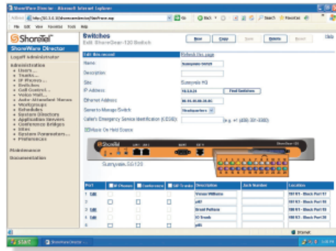
Figure 1: Graphical installation capabilities make it easy for new switches to be automatically added to the network.
